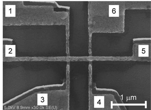
Fig. 1. Scanning electron microscope (SEM) image of fabricated lateral spin valve device.
