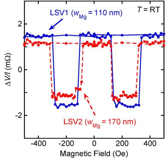
Fig. 3. Field dependence of nonlocal spin valve signal at room temperature for devices with different Mg wire widths and injector-detector separation of 250 nm.
