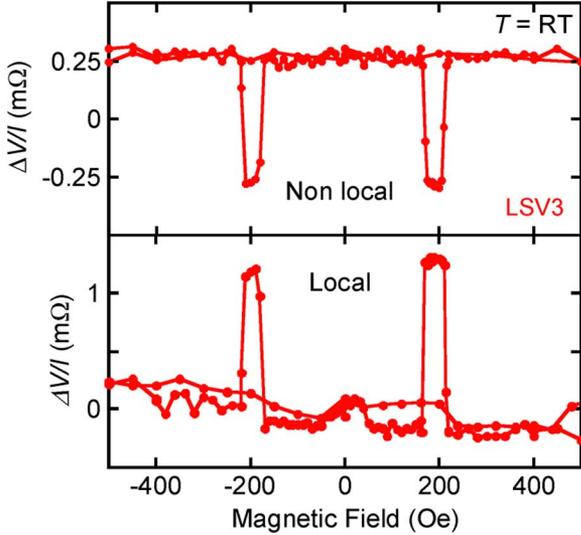
Fig. 2. Field dependence of nonlocal and local spin valve signals at room temperature for device with injector-detector separation of 400 nm.
