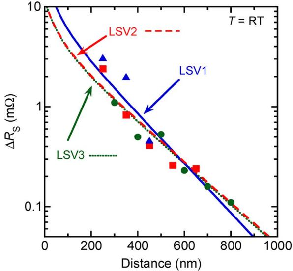
Fig. 4. Injector-detector separation dependence of nonlocal spin valve signal  $\Delta R_S$  for devices with different Mg and Py wire widths. Lines are fitted curves using eq. (1).
