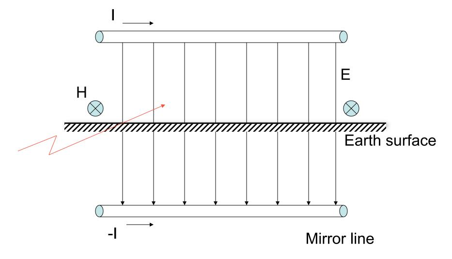
Electric and magnetic fields are produced between two lines
