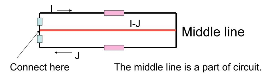
Arrange electric loads symmetrically around the middle line. (Decouple normal and common modes.)
