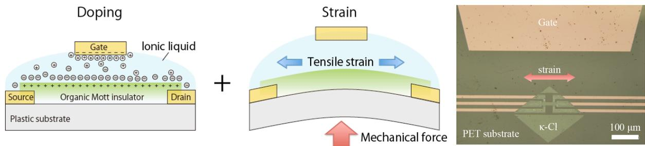
Fig. 1. Schematic side view and optical top view of the organic Mott EDLT based on  $\kappa$ -Cl. A gate voltage varies doping and a strain modifies the effective pressure in the same sample.
