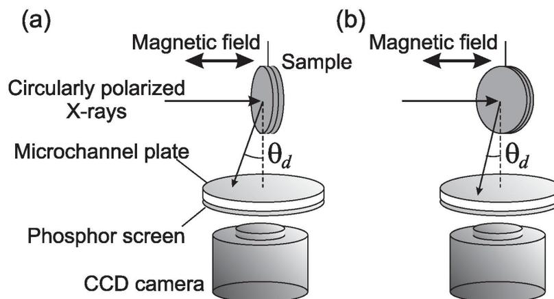
Fig. 1: Schematic diagram of the depth-resolved X-ray magnetic circular dichroism technique at normal (a) and grazing (b) X-ray incidence. The emitted electrons are collected with an imaging type detector at different detection angles, which determine the probing depths.
