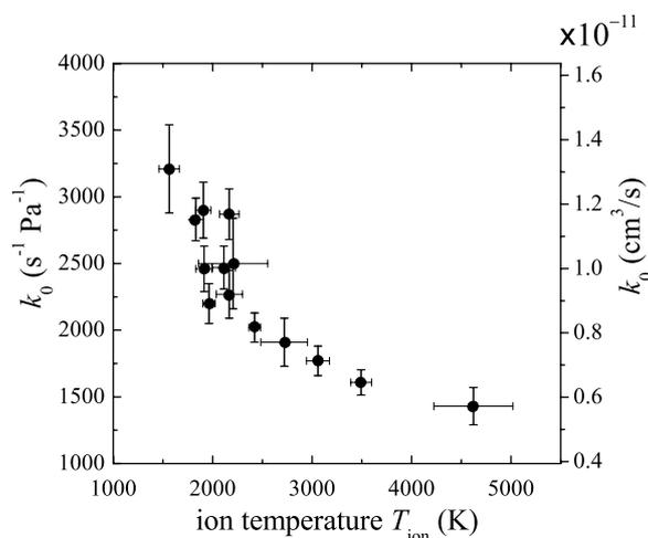
**Figure 13.** Dependence of the reaction rate coefficient of  $\text{Ca}^{+*}(\text{D}_J) + \text{H}_2\text{O} \rightarrow \text{products}$  on  $\text{Ca}^+$  ion temperature. The ion temperature was evaluated by the Doppler widths of the LIF spectra measured at the start and end of each series of measurements.
