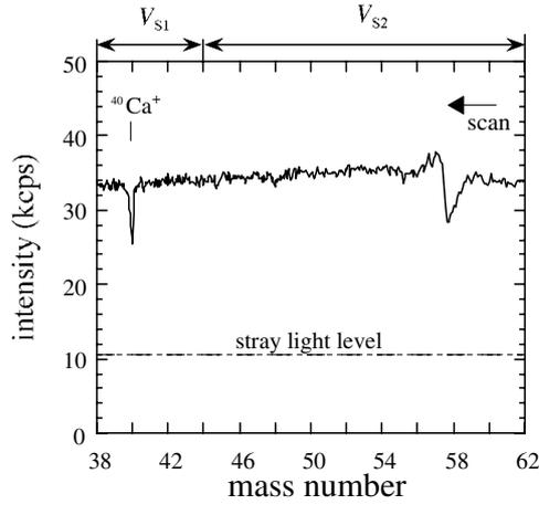
**Figure 6.** Signal of the reaction-product ions strengthened by introduction of H<sub>2</sub>O. The reaction time corresponding to the IR laser-off period was set at 60 s. Experimental parameters: the perturbation amplitude was set at  $V_{S2} = 5.0$  mV for  $M = 57, 58$  and at  $V_{S1} = 0.4$  mV for  $M = 40$ .  $I_V = 72 \mu\text{W}$ ,  $I_{IR} = 1.8$  mW. The H<sub>2</sub>O pressure was  $1.1 \times 10^{-6}$  Pa. The other parameters were the same as presented in figure 5.
