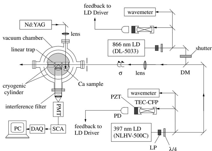
**Figure 1.** Experimental set-up. LD: laser diode, LP: linear polarizer,  $\lambda/4$ : quarter-wave plate, DM: dichroic mirror, PD: photodiode, PZT: piezoelectric actuator, TEC-CFP: temperature-stabilized confocal Fabry–Perot, DAQ: data acquisition card, SCA: single-channel analyser, PMT: photomultiplier tube.
