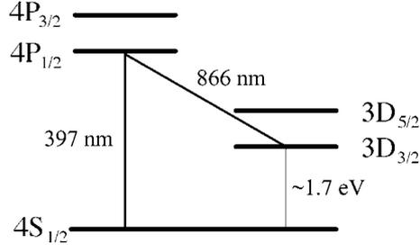
**Figure 2.** Simplified energy level diagram of  $^{40}\text{Ca}^+$  (not to scale).
