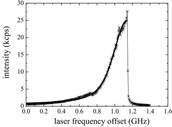
**Figure 3.** Laser cooling spectrum of trapped  $^{40}\text{Ca}^+$  ions. The thick curve is obtained by fitting the Voigt profile to part of the spectrum data. The estimated half-width of the Gaussian part is 187 MHz (HWHM). The experimental parameters are: rf  $f_{\text{rf}} = 3.222$  MHz, rf voltage  $V_{\text{ac}} = 150$  V. The violet and IR lasers were set at  $I_{\text{V}} = 15 \mu\text{W}$  and  $I_{\text{IR}} = 2.6$  mW, respectively.
