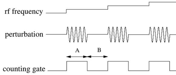
**Figure 4.** The time sequence of the LIF mass spectroscopy. Periods A (heating time) and B (cooling time) were set at 0.1–1.0 s to optimize the observation.
