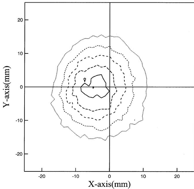
Fig. 2. 2D position distribution of  $H^+$  sputtered by 700 eV  $Xe^{7+}$  with the incident angle 45 degrees at the moment of the surface impact.
