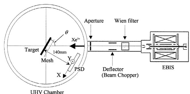
Fig. 1. A schematic diagram of the experimental setup.
