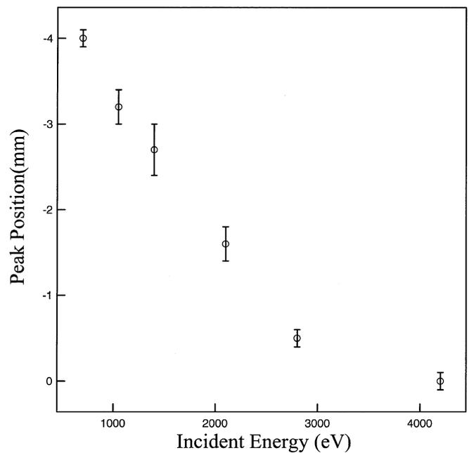
Fig. 4. Sputtered  $H^+$  peak position in the  $X$  direction as a function of the incident energy of  $Xe^{7+}$ . Incident angle with respect to the target normal at the moment of the surface impact was 45 degrees regardless of the incident energy.
