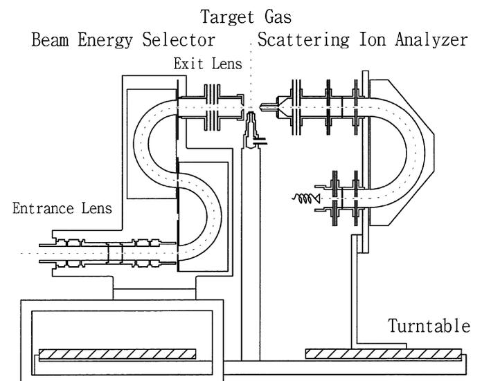
Fig. 1. Schematic view of the experimental apparatus installed in the collision chamber.
