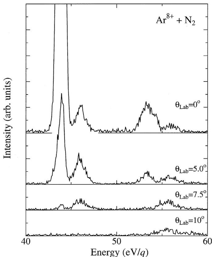
Fig. 2. Energy distributions of scattered ion (Ar<sup>8+</sup>, Ar<sup>7+</sup>, and Ar<sup>6+</sup>) for 36.6 eV/q (7.3 eV/u) Ar<sup>8+</sup>-N<sub>2</sub> collisions at scattering angles as indicated.
