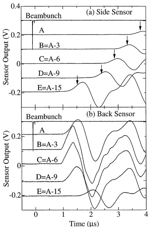
Fig. 1. Elastic waveforms observed at the side sensor (a) and back sensor (b) on Al sample along with the beam-bunch signal by the fast monitor. A–E denote the waveforms for different beam-spot positions. Arrows in (a) show the expected arrival time of the longitudinal wave to the side sensor.
