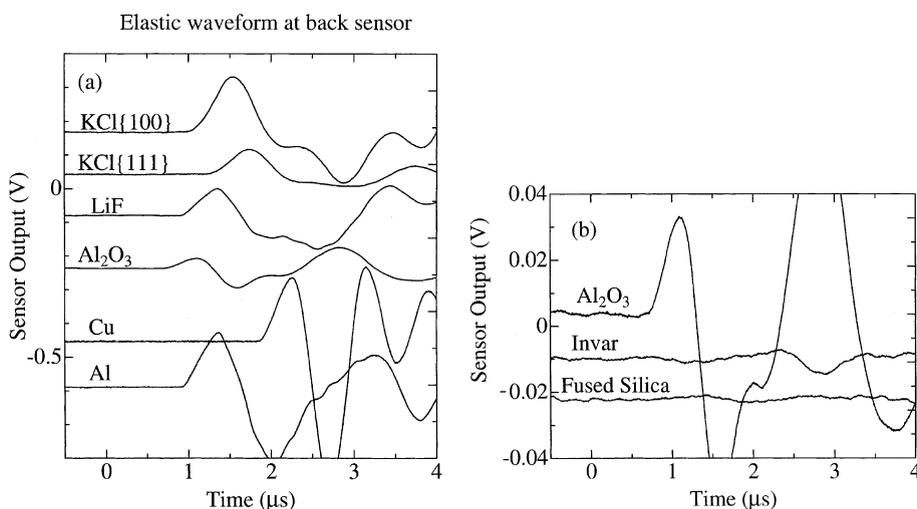
Fig. 2. Elastic waveforms captured by a sensor opposite to the beam spot. The waveforms are normalized to the beam-bunch intensity. The ordinate is expanded by a factor of 10 in (b).
