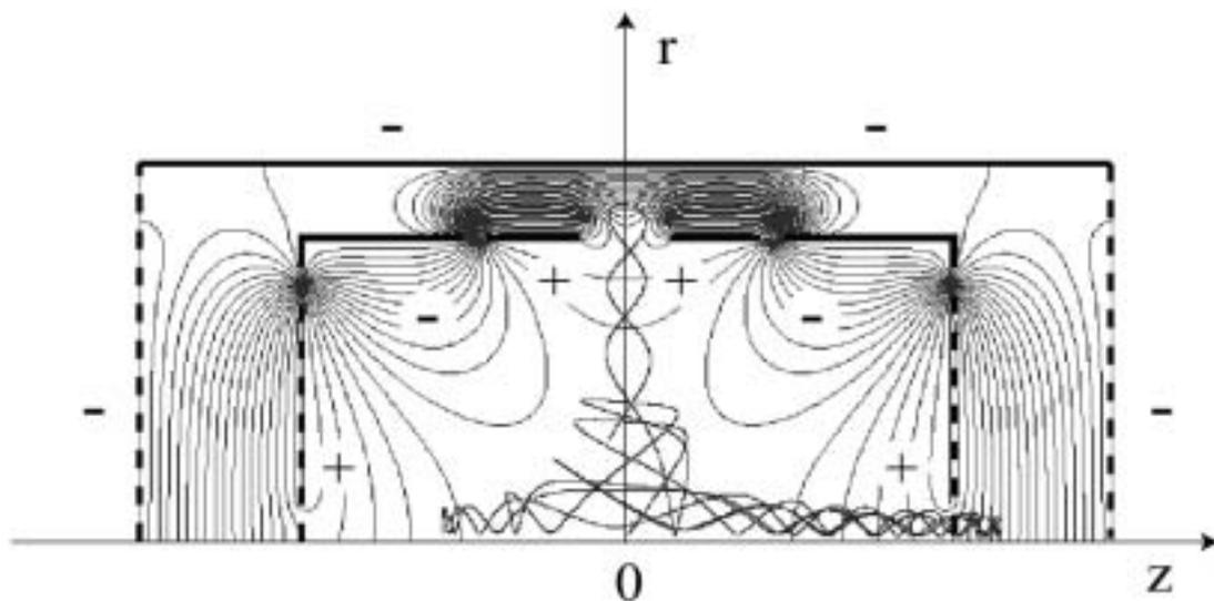
Fig. 3. Electrode configuration for the octupole electric field formation for positron trapping and the outer electrodes for hot antiproton confinement (symmetric with respect to the axis  $z$ ). The solid lines show the equi-potential lines in and outside the MECO. An example of the trajectories of 30 eV antiprotons is also given.
