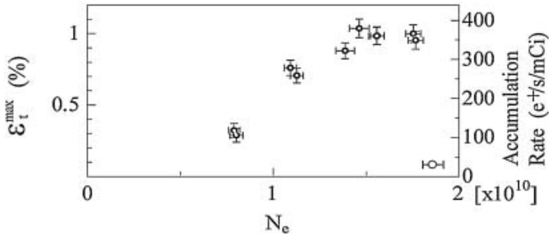
Fig. 6. The optimized trapping efficiency as a function of the total electron number in the electron plasma. The right vertical scale gives the accumulation rate normalized by the  $^{22}\text{Na}$  positron source intensity [47].
