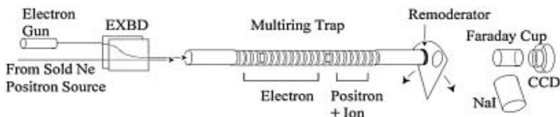
Fig. 5. A schematic diagram of the experimental setup for the UHV compatible positron accumulation (See the text for details). [47]
