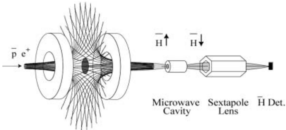
Fig. 2. A schematic layout of the cusp trap configuration (the left half) together with a microwave cavity and a magnetic sextupole lens for hyperfine transition measurements.
