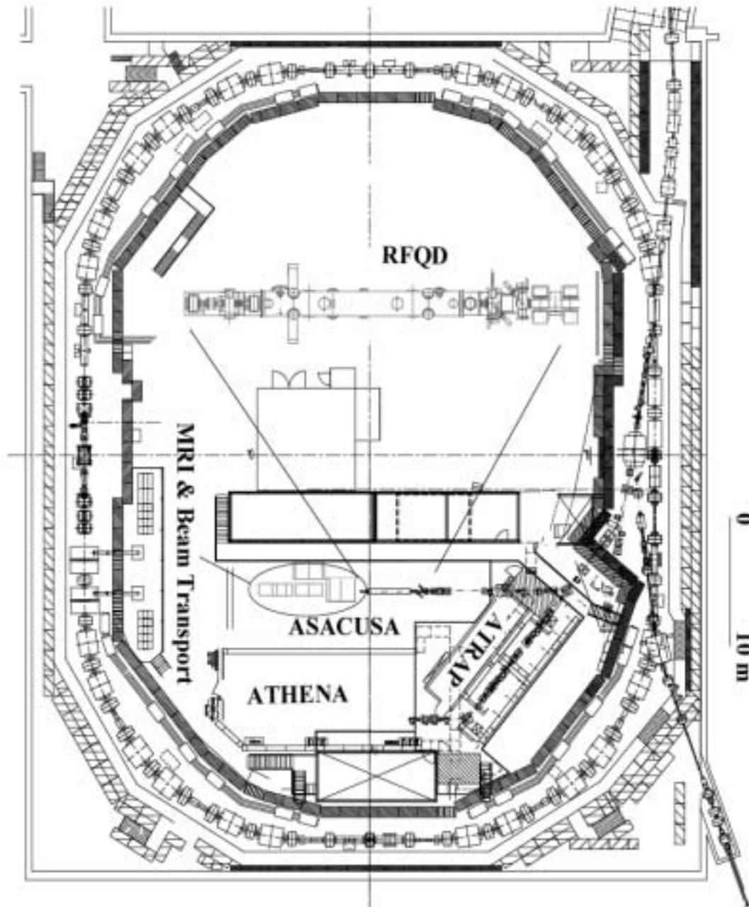
Fig. 1. A schematic layout of AD, ASACUSA, ATHENA, and ATRAP. A magnified view of the RFQD is shown in the left half of AD.
