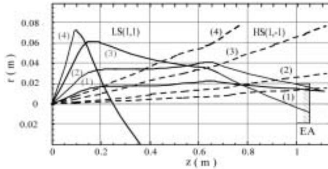
Fig. 4. The solid lines are the trajectories of 0.268 meV  $\bar{H}$  atoms in LS(1,1) state with emission angles  $q = (1) 5^\circ$ , (2)  $10^\circ$ , (3)  $20^\circ$ , and (4)  $30^\circ$ . The dotted lines are those of 0.268 meV  $\bar{H}$  atoms in the HS(1, -1) state with the emission angle  $q = (1) 0.5^\circ$ , (2)  $1.1^\circ$ , (3)  $3^\circ$ , and (4)  $5^\circ$ . The EA indicates the entrance aperture of the microwave cavity.
