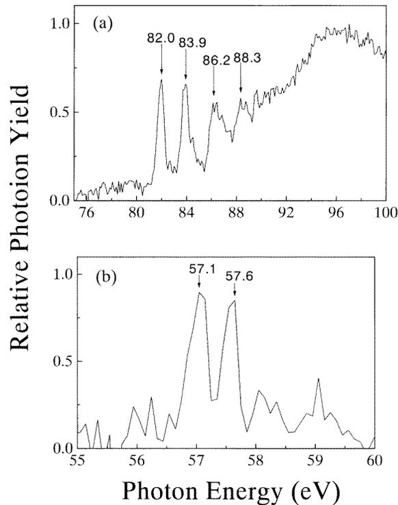
**Figure 2.** The detailed structures in the photoion-yield spectrum of Xe<sup>2+</sup> (see figure 1(c)). Data points were acquired in 0.1 eV steps. The energies of several prominent peaks are determined in eV as shown above the arrows. (a) The spectrum around 90 eV, obtained with high-energy resolution. (b) The spectrum below 60 eV with low-energy resolution.
