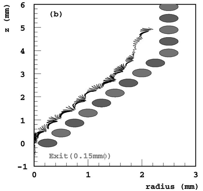
Fig. 2. Typical ion trajectory in the RF ion-guide.
