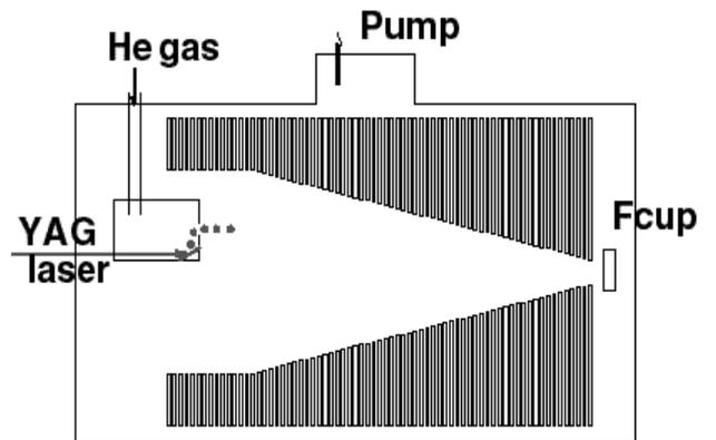
Fig. 3. Test RF ion-guide gas cell.
