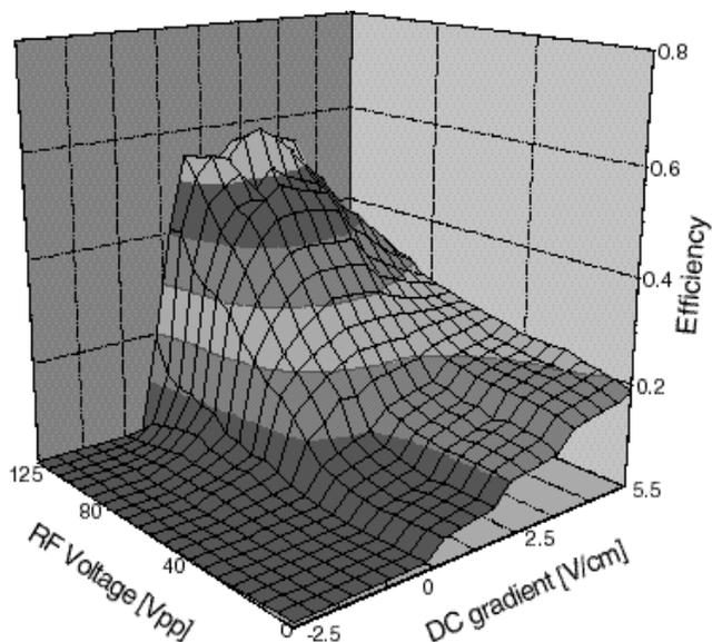
Fig. 4. Experimental result of ion transport in the RF ion-guide.
