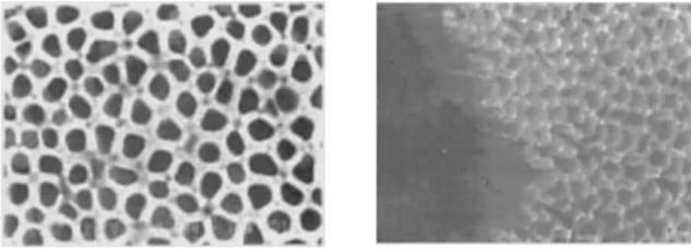
Fig. 2. Picture of microcapillary foil. Top view (left) and a side view (right) are shown.
