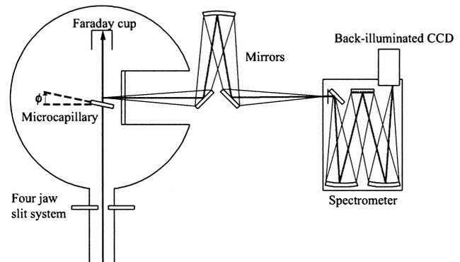
Fig. 1. Schematic drawing of the experimental setup.
