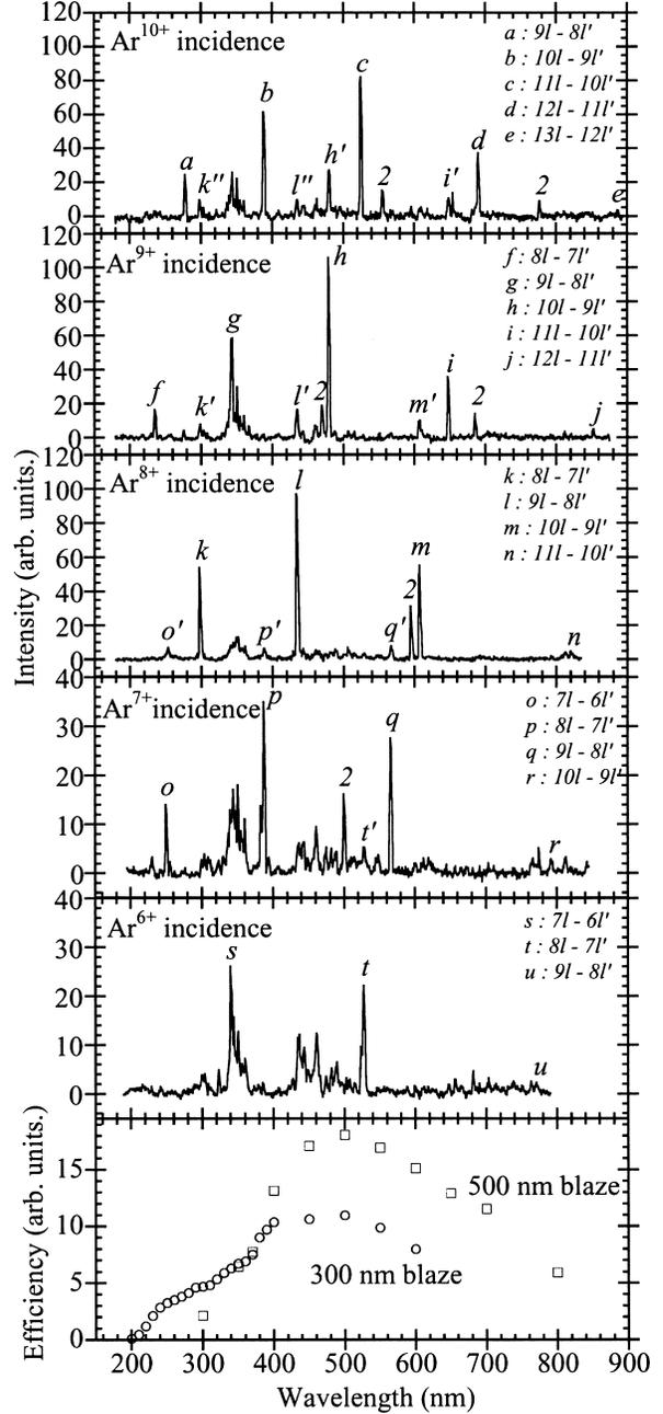
Fig. 3. Observed spectra for  $\text{Ar}^{Q+}$  ( $6 \leq Q \leq 10$ ) incident ions and relative efficiency curves of the detection system.
