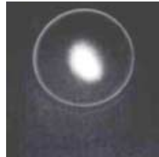
Figure 3: Positron beam profile observed by an MCP. The MCP active diameter is 10mm.
