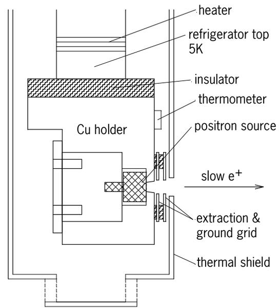
Fig. 3. Drawing of the positron source assembly.
