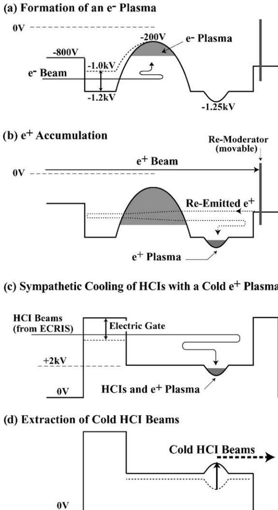
Fig. 1. (a)–(d) Schematic descriptions of the HCI trapping, cooling and extraction.
