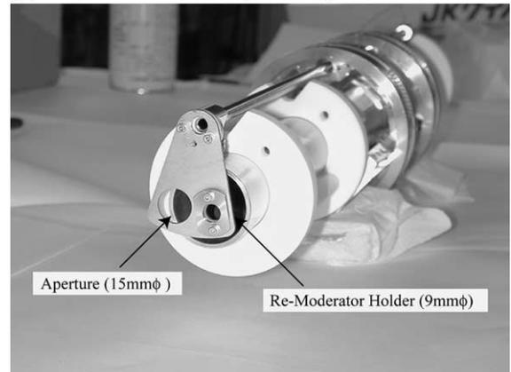
Fig. 3. Photos of (a) the MRT and (b) the re-moderator holder.
