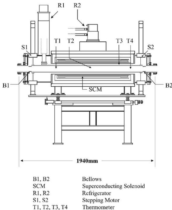
Fig. 2. A schematic drawing of the 5 T superconducting solenoid and the UHV vessel.
