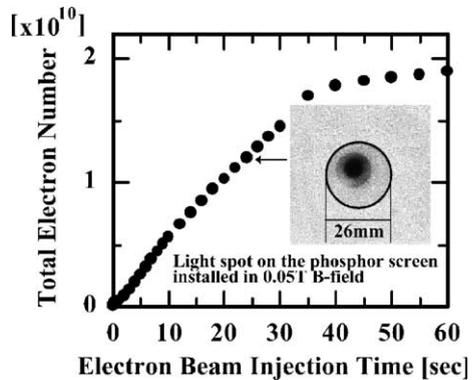
Fig. 4. The number of trapped electrons as a function of the electron injection time for an electron beam of 1  $\mu\text{A}$ . The inset shows the CCD image of the extracted plasma at  $B = 0.05$  T.
