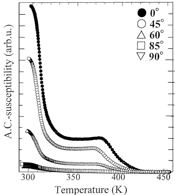
Fig. 4. Temperature dependence of AC-susceptibility for Fe-30.2at.%Ni Invar alloy after irradiated with 100 MeV Xe to the dose of  $10^{14}$  ions/cm<sup>2</sup>. The angles shown are between the surface of the specimen and the direction of external field.
