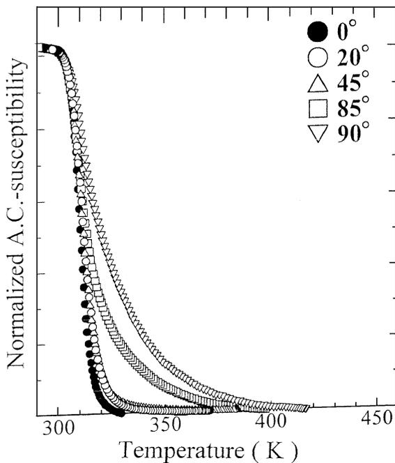
Fig. 3. AC-susceptibility versus temperature curves for Fe-30.2at.%Ni Invar alloy before irradiation in normalized scale at  $T = 300$  K and  $\theta = 0$ .
