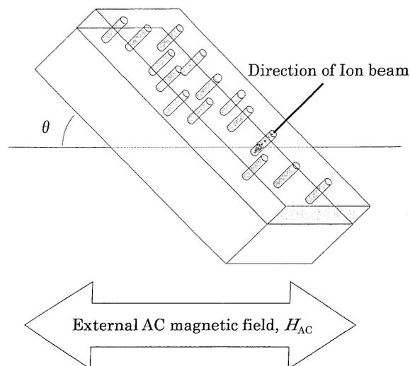
Fig. 1. Schematic illustration of a square plate specimen irradiated by 100 MeV Xe ions and the direction of external AC-magnetic field.
