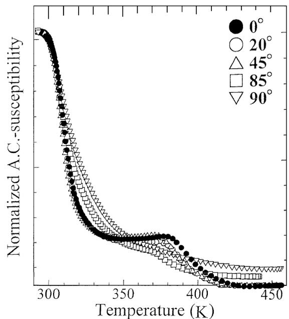
Fig. 5. AC-susceptibility versus temperature curves for Fe-30.2at.%Ni Invar alloy after the irradiation in normalized scale at  $T = 300$  K and  $\theta = 0$ .
