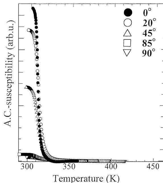
Fig. 2. Temperature dependence of AC-susceptibility for Fe–30.2at.%Ni Invar alloy before irradiation: The angles shown are between the surface of the specimen and the direction of external field.
