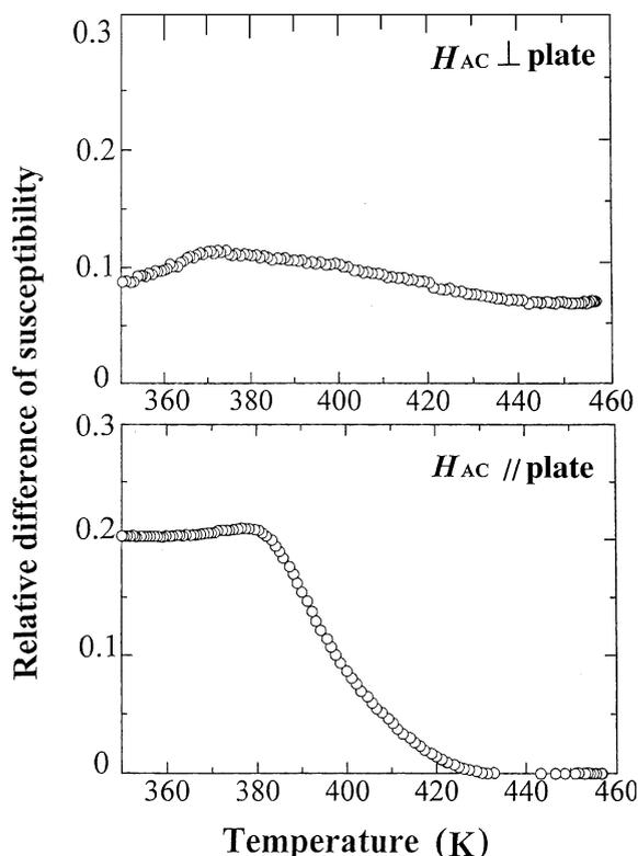
Fig. 6. Temperature dependence of the differences of AC-susceptibility between before and after the irradiation in normalized scale.
