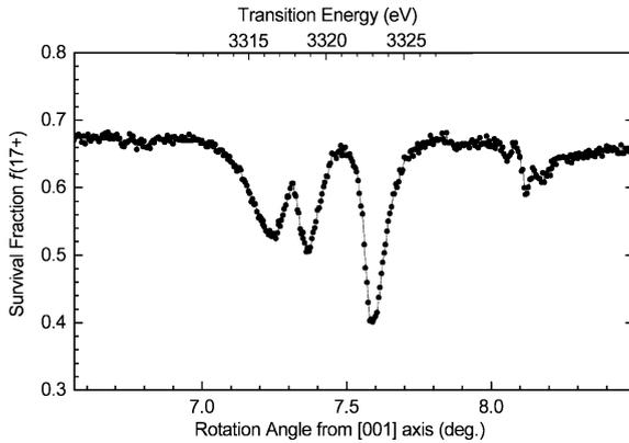
Fig. 2. Survival fraction  $f(17+)$  around the resonance condition for  $(k, l) = (3, 1)$  as a function of the rotation angle from  $[001]$  axis. The corresponding transition energy for the  $(k, l) = (3, 1)$  resonance is shown in the upper scale. The small dip around  $8.1^\circ$  is thought to correspond to the resonance with  $(k, l) = (4, -4)$ .
