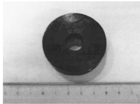
FIG. 4. A photo of the superconductor ring used in the High- $T_C$  EBIS. A ruler in centimeter units is also shown.
