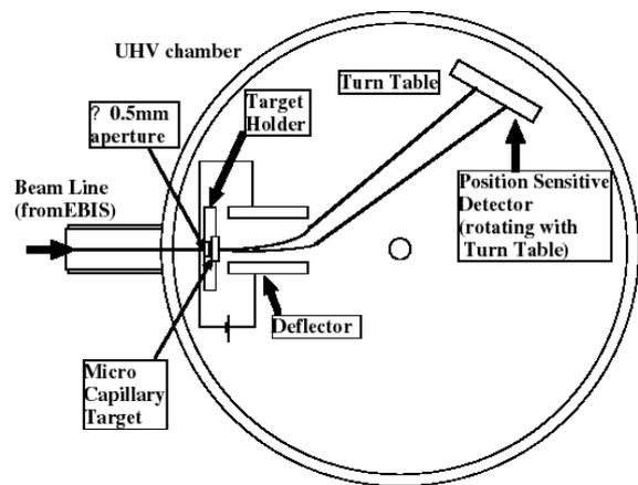
Fig.1: Experimental set up for charge state analysis
