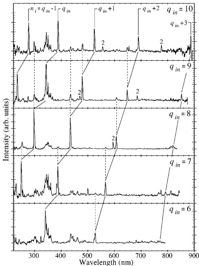
FIG. 1. Wide-range spectra for 2.0keV/amu  $\text{Ar}^{q_{in}+}$  incident ions. Lines connected by the solid lines are attributed to  $\Delta n=1$  transitions of  $\text{Ar}^{(q_{in}-1)+}$ . The solid lines connect transitions with  $n_i=q_{in}+s$  among different  $q_{in}$  for a fixed  $s$ . Second-order reflections are marked by 2.
