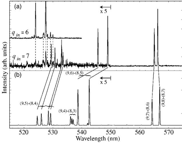
FIG. 2. (a) High-resolution spectra around  $n_i=9$  transitions of  $\text{Ar}^{6+}$  ( $q_{in}=7$ ) and  $n_i=8$  transitions of  $\text{Ar}^{5+}$  ( $q_{in}=6$ ) ions. (b) A spectrum generated using results by MCHF codes. Lines identified are connected by the solid lines.
