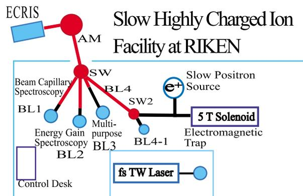
Fig. 1. Layout of the facility. HCI beams from the ECRIS are delivered to three experimental setups(BL1 to 3) and to the HCI trap(BL4). AM: analyzing magnet, SW, SW2: switching magnet. The BL4-1 is now under preparation for the BCS experiment. AM, SW, SW2, and beam lines indicated by red color can be floated.
