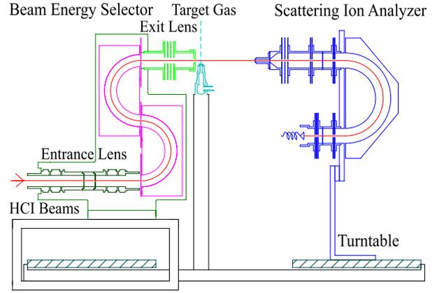
Fig. 3. Energy selector and scattering ion energy analyzer at the BL2. Decelerated HCIs are energy selected and collide with the gas target. After the collisions, the energy and scattering angle of the HCIs are measured by the scattering ion energy analyzer.
