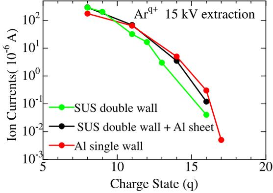
Fig. 2. Argon ion currents from the ECRIS measured after AM with different plasma chamber. Extraction voltage is 15 keV. Beam size at Faraday cup is 18 mm  $\times$  18 mm. Green, black, and red circles are for the SUS double wall chamber, the SUS double wall chamber with the Al sheet, and the Al single wall chamber, respectively.
