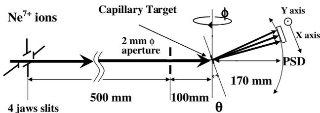
Fig. 1. Experimental setup.  $\text{Ne}^{7+}$  ions are collimated by 4 jaws-slits and a 2 mm  $\phi$  aperture before the target, which can be rotated to the  $\theta$  and  $\phi$  directions as indicated. Transmitted ions are measured by a 2-D position sensitive detector (PSD). An electrostatic deflector can be set just after the target for analyzing the charge state of the transmitted ions.
