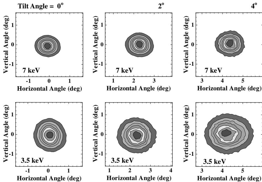
Fig. 4. 2-D images of transmitted 3.5 and 7 keV  $\text{Ne}^{7+}$  ions after intensity saturation for different tilt angles. The target was tilted to the  $\theta$  direction and  $\phi = 0^\circ$  for all cases. The charge state of the transmitted ions was not analyzed. Contours are plotted in linear scales.
