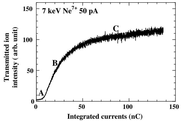
Fig. 2. Intensity evolution of 7 keV  $\text{Ne}^{7+}$  ions. The capillary target was set at the angles  $\theta = 2^\circ$  and  $\phi = -1^\circ$  from the previous angles  $\theta_0 = 2^\circ$ ,  $\phi_0 = 1^\circ$ . A, B and C indicate the ranges corresponding to the 2-D images in Fig. 3.
