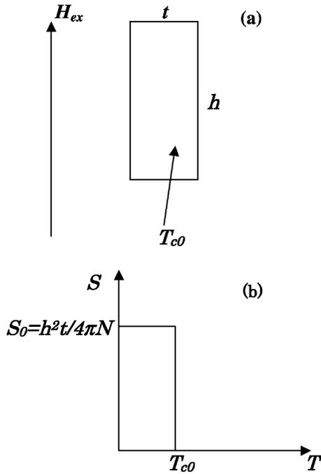
Fig. 1. (a) Distribution of  $T_c$  in the specimen before irradiation and (b) temperature dependence of the slope of  $M-H_{ex}$  curve,  $S$ . Direction of magnetic field is also shown.
