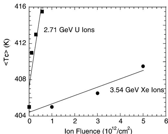
Fig. 5. Mean value of Curie temperature,  $\langle T_c \rangle$ , as a function of ion-fluence for Xe ion irradiation and U ion irradiation.
