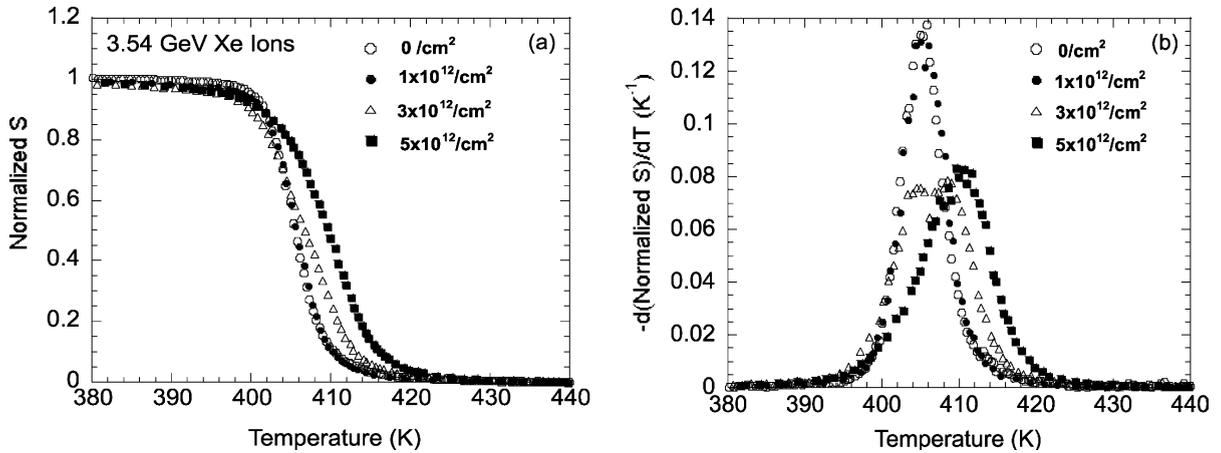
Fig. 3. Temperature dependence of the slope of  $M-H_{ex}$  curves,  $S$ , for 3.54 GeV Xe ion irradiation (a) and their temperature derivatives (b).
