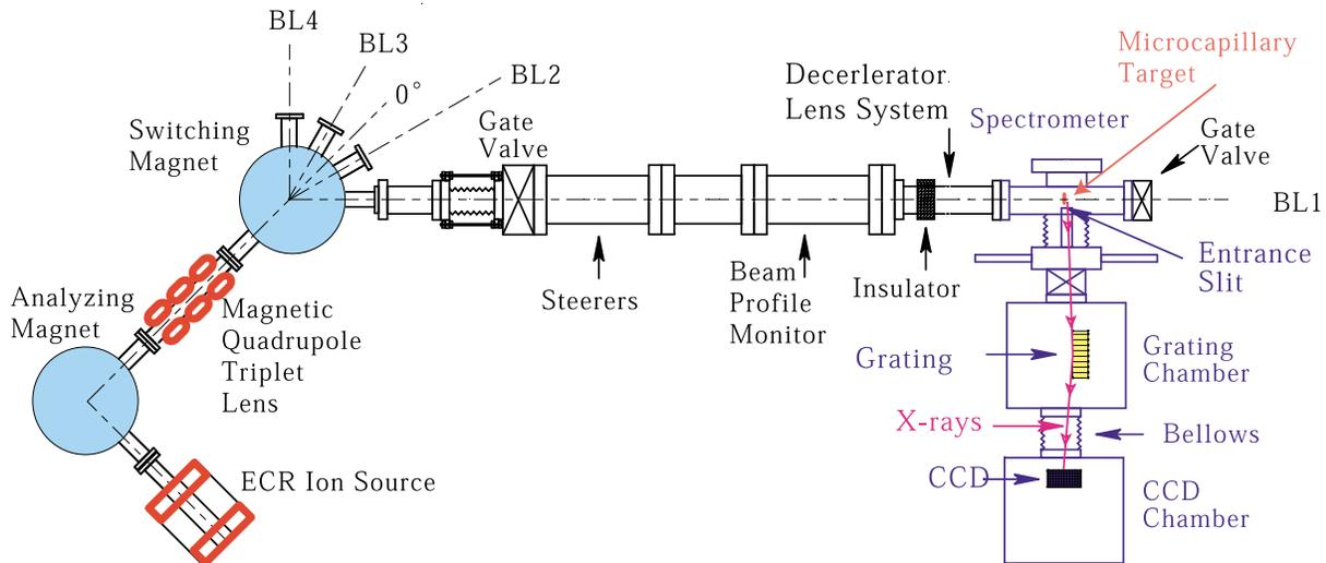
Fig. 1. Schematic drawing of experimental configuration.
