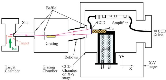
Fig. 3. Schematic drawing of the high-resolution soft X-ray spectrometer.
