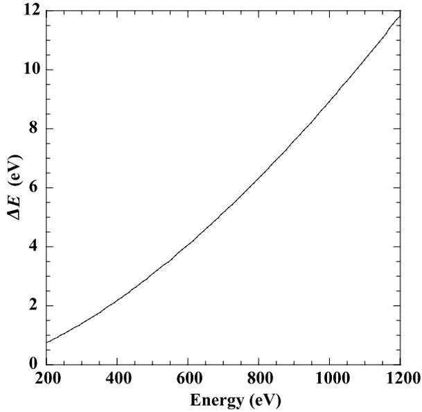
Fig. 6. Energy resolution (FWHM) dependences on X-rays energy of the spectrometer.
