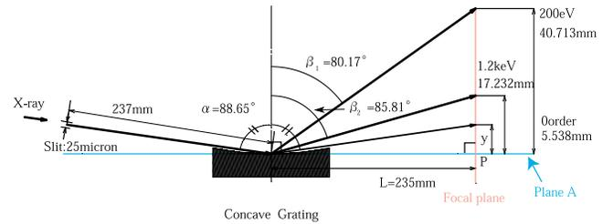
Fig. 4. Schematic drawing of the characteristic optical path of the grating for soft X-ray with the focal plane.
