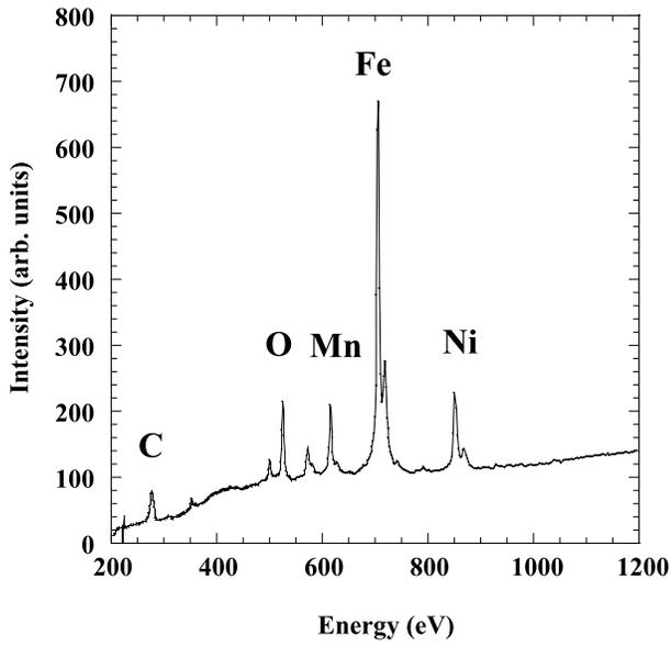
Fig. 5. Spectrum of stainless steel target with 4 keV electron impact, measured with the spectrometer.
