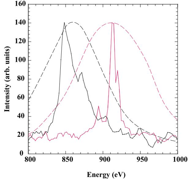
Fig. 7. Spectra of  $K$  X-rays measured with the spectrometer, for 2.3 keV/u  $\text{Ne}^{9+}$  ions transmitted through a Ni capillary (red solid line), and those hit with a stainless steel plate (black solid line). Spectra of  $K$  X-rays measured with Si(Li) detector, for 9 keV/u  $\text{Ne}^{9+}$  ions transmitted through a Ni capillary (red dashed line), and those hit with an Al plate (black dashed line) are shown for comparison.
