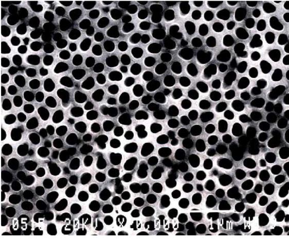
Fig. 2. Image of Ni microcapillary (taken by SEM).
