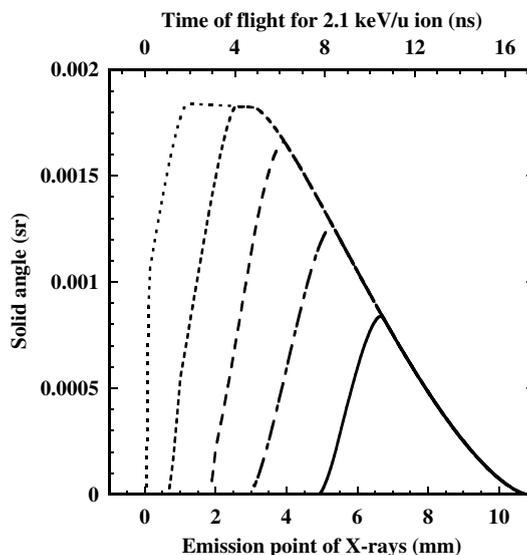
Fig. 2. Solid angle subtended by the Si(Li) X-ray detector as a function of position  $z$  for the shield positions of 0 mm (dotted line), 1 mm (short-dashed line), 2 mm (long-dashed line), 3 mm (dot-dashed line), and 4 mm (solid line). The  $z$ -axis is the along the ion beam and the origin is at the microcapillary target position. The time of flight for 2.1 keV/u ions is shown in the top.
