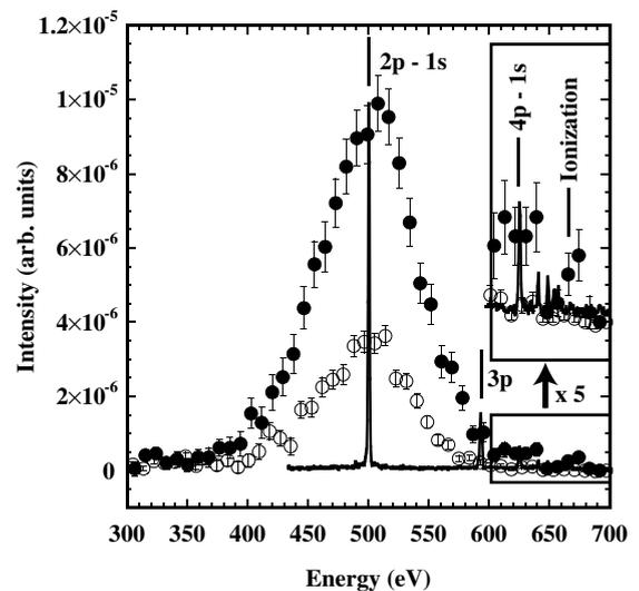
Fig. 4. Energy spectra of N K X-rays with  $(q_i, q_f) = (7, 6)$  for shield positions of 0 mm (●) and 1 mm (○). A spectrum of X-rays measured with a high-resolution soft X-ray spectrometer at immediately downstream of the Ni microcapillary target for 2.3 keV/u  $N^{7+}$  incidence was shown by solid line for comparison [11]. The bars with transition terms show transition energies [17].
