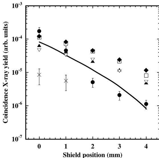
Fig. 3. The integrated coincidence X-ray yields as a function of the shield position for incident and final charge state combinations  $(q_i, q_f)$  of  $(7, 6)$  (●),  $(7, 5)$  (◆),  $(7, 4)$  (▲),  $(6, 5)$  (□),  $(6, 4)$  (▽) and  $(6, 3)$  (×). The solid line shows the integrated K X-ray yield obtained via cascade calculation of one electron (H-like) ion initially populated according to the report of visible light measurement [8], considering the solid angle calculation (Fig. 2).
