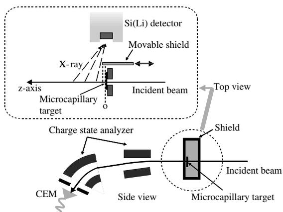
Fig. 1. Schematic drawing of the experimental setup.
