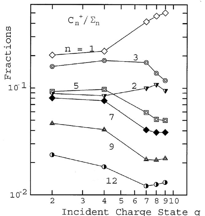
Fig. 3. Intensity ratios between  $C_n^+$  and  $\Sigma_n$  as a function of  $q$ .
