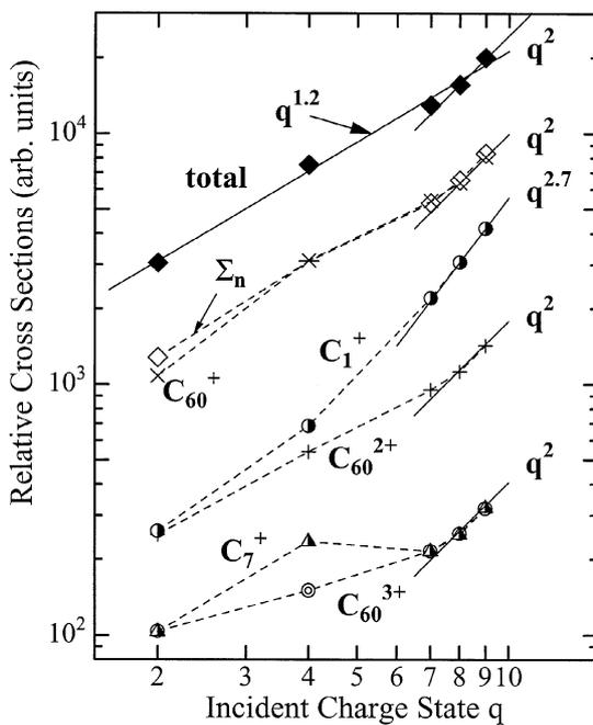
Fig. 2. Cross sections for various product ions as a function of the projectile charge state  $q$ . The symbol  $\Sigma_n$  represents the sum of cross sections over small fragment ions  $C_n^+$  of  $n = 1 \sim 12$ , and “total” is the total cross sections of all product ions.
