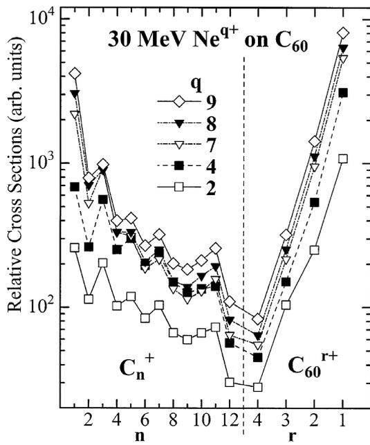
Fig. 1. Cross sections for the production of fragment ions  $C_n^+$  and intact ions  $C_{60}^{r+}$  as a function of  $n$  or  $r$ .
