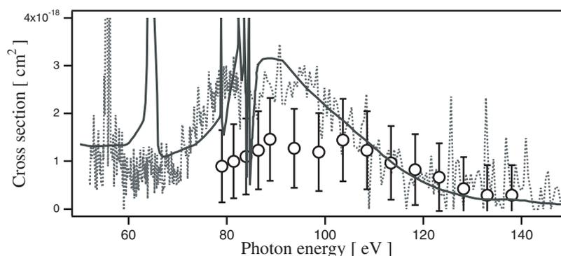
**Figure 3.** Comparison of the single-photoionization cross sections for  $\text{Xe}^+$  obtained experimentally and theoretically. Absolute measurements (O), relative measurements (- - -), theoretical results reported by Amusia *et al* [20] (—).
