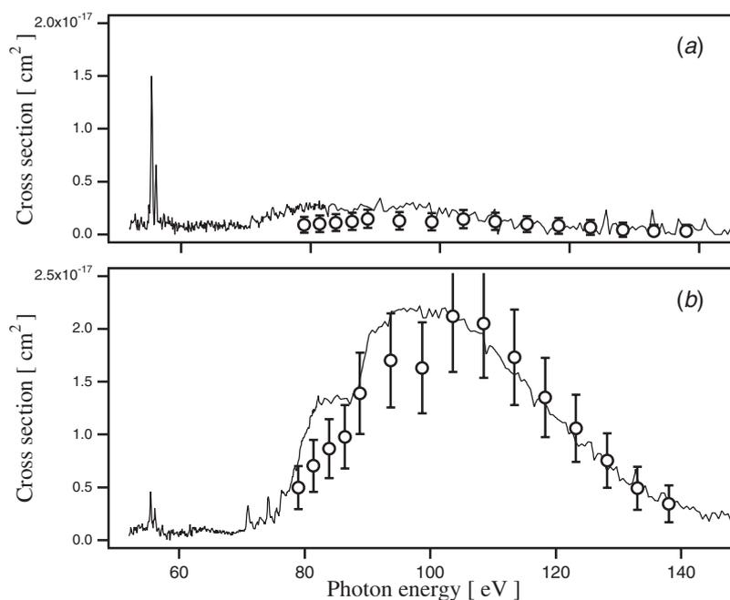
**Figure 2.** (a) Absolute single-photoionization cross sections and (b) double-photoionization cross sections for Xe<sup>+</sup>. Absolute measurements (○), relative measurements (—). The sum of the relative cross sections was normalized to the absolute total cross section at 103.6 eV.
