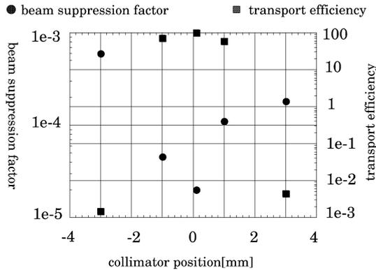
Fig. 2. The measured beam suppression factor with  $^{20}\text{Ne}^{7+}$  beam. The horizontal axis shows the vertical position of the 4 mm  $\varnothing$  collimator at the target chamber. RMS was tuned for  $\Delta M = 1$  heavier ions than the beam.
