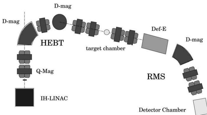
Fig. 1. The ion optical configuration from the linac to a detector system. At the downstream of a target chamber, there is a recoil mass separator.
