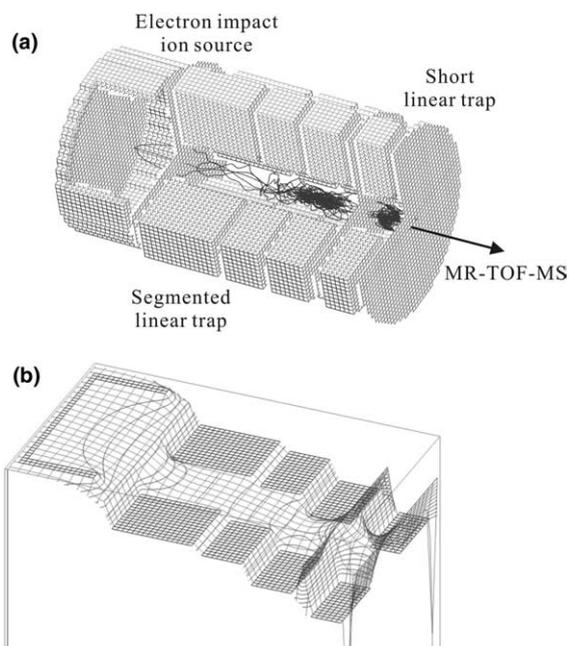
Fig. 1. (a) Calculated trajectories of singly charged ions of mass 100 and (b) the DC potential distribution in the linear trap as determined by SIMION.
