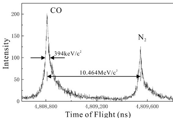
Fig. 2. The obtained mass spectrum of the CO–N<sub>2</sub> mass doublet after 641 laps.
