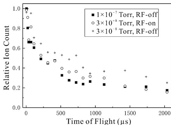
Fig. 3. The recorded ion intensity as a function of ion flight time relative to the intensity after one pass. Squares and crosses denote the ion count rate at residual gas pressures of  $1 \times 10^{-7}$  Torr as well as  $3 \times 10^{-8}$  Torr with no RF power being applied to the ion trap while the ions were flying in the MR-TOF-MS. Circles denote the ion count rate at  $3 \times 10^{-8}$  Torr when RF power was applied which locally increased the residual gas pressure.
