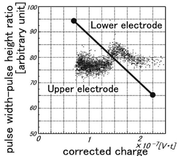
Fig. 5. Scatter plot of a ratio of pulse width to pulse height as a function of corrected charge which is proportional to the energy for  $\text{Ne}^{7+}$  ions.
