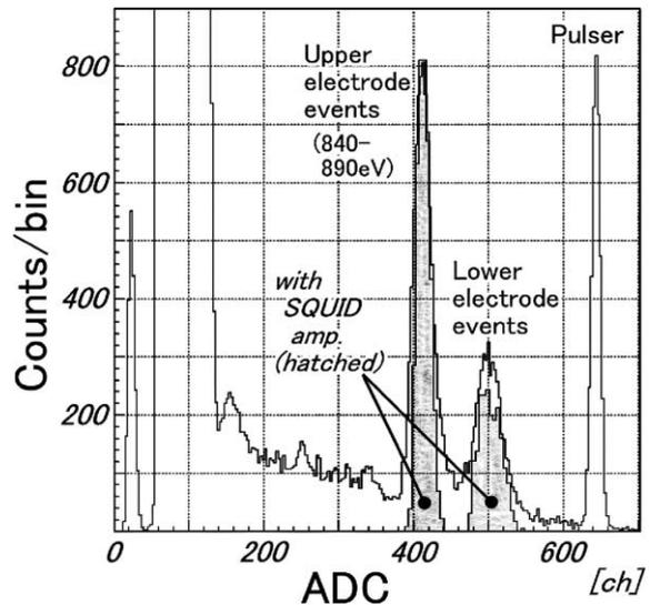
Fig. 4. Energy spectrum of  $\text{O}^{7+}$  K X-rays.
