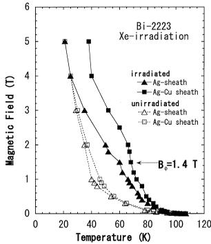
Fig. 1. The irreversibility temperature are plotted in  $H$ - $T$  plane for the Ag and Ag-Cu alloy sheathed Bi-2223 tapes with columnar defects by solid symbols and for the unirradiated ones by open symbols, respectively.
