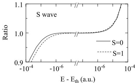
FIG. 5. The accuracy of the fitting of Baz's formula (3) to the calculated  $S$ -wave singlet (full curve) and triplet (broken curve) annihilation cross sections. The ratio of the fitted Baz' formula to the calculated results is plotted against the incident positron energy  $E$  measured from the threshold  $E_{\text{th}}$  for the production of positronium.
