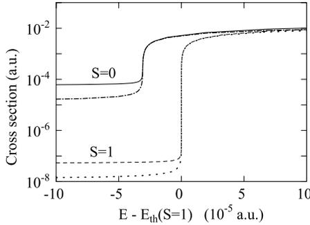
FIG. 1. The singlet ( $S=0$ ) and triplet ( $S=1$ ) annihilation cross sections  ${}^{1,3}\sigma$  (full and broken curves) and their  $S$ -wave components  ${}^{1,3}\sigma_0$  (dot-dashed and dotted curves) plotted as functions of the incident positron energy  $E$  measured from the threshold  $E_{\text{th}}(S=1)$  of the formation of an ortho(triplet)-positronium. The total annihilation cross section for an unpolarized positron beam is calculable by  $({}^1\sigma + 3{}^3\sigma)/4$ .
