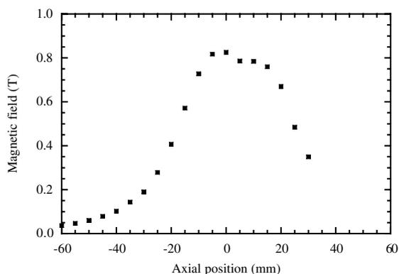
Fig. 2. Distribution of trapped magnetic field at 77 K.
