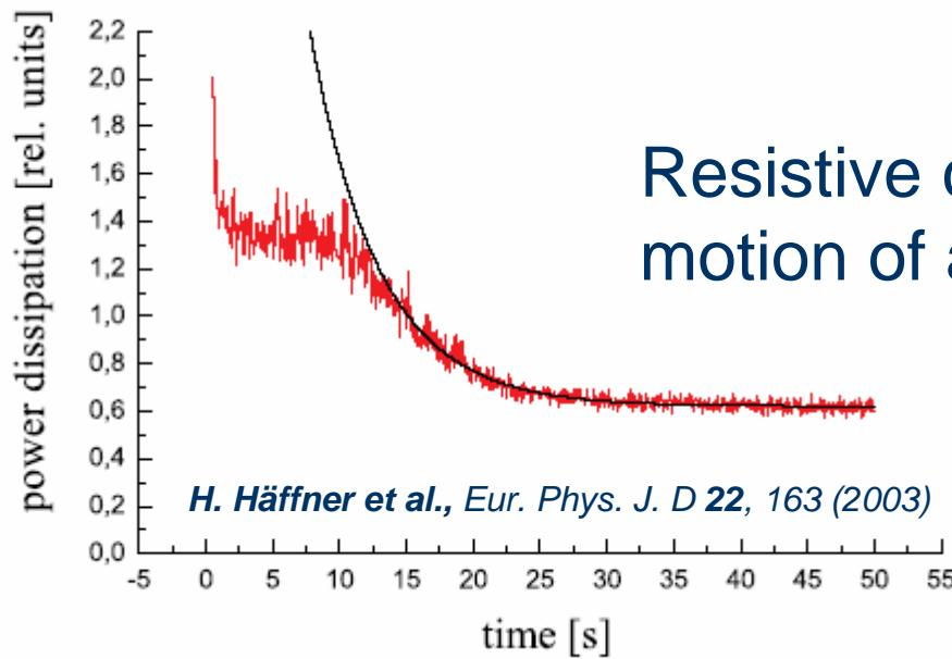
Resistive cooling of the axial motion of an ion cloud ( $^{30} \text{C}^{5+}$ )
