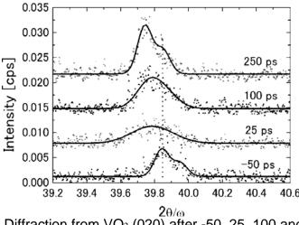
Time-resolved XRD Diffraction from  $VO_2$  (020) after -50, 25, 100 and 250 ps. The dramatic change in the diffraction spectra indicates phase transition of the crystal.
