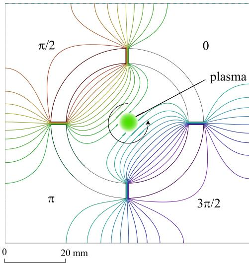
FIG. 6. Cross sectional view of the segmented electrode HE4 for applying a rotating wall. Equipotential lines are also shown.
