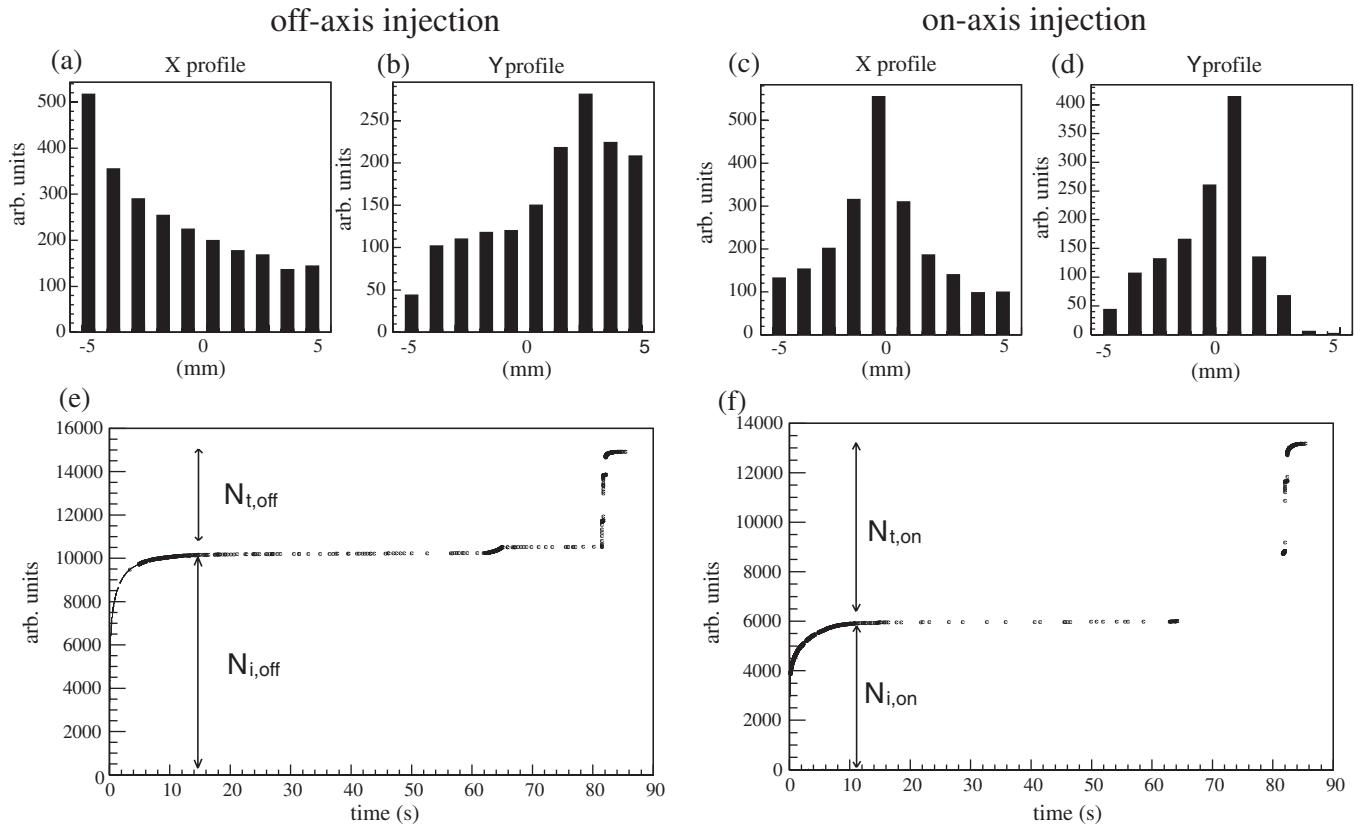
FIG. 14. (a), (b) Injected  $\bar{p}$  beam  $x/y$ -projected profiles read by the foil detector, respectively, and (e) is the annihilation count of  $\bar{p}$  for the off-axis injection case. Parts (c), (d), and (f) are in the case of on-axis injection.
