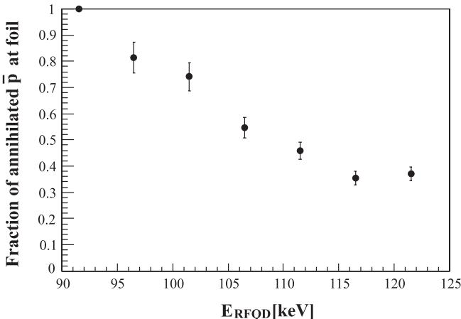
FIG. 12. Annihilated fraction of RFQD-decelerated  $\bar{p}$  beam in the PET foil against their injection energy.
