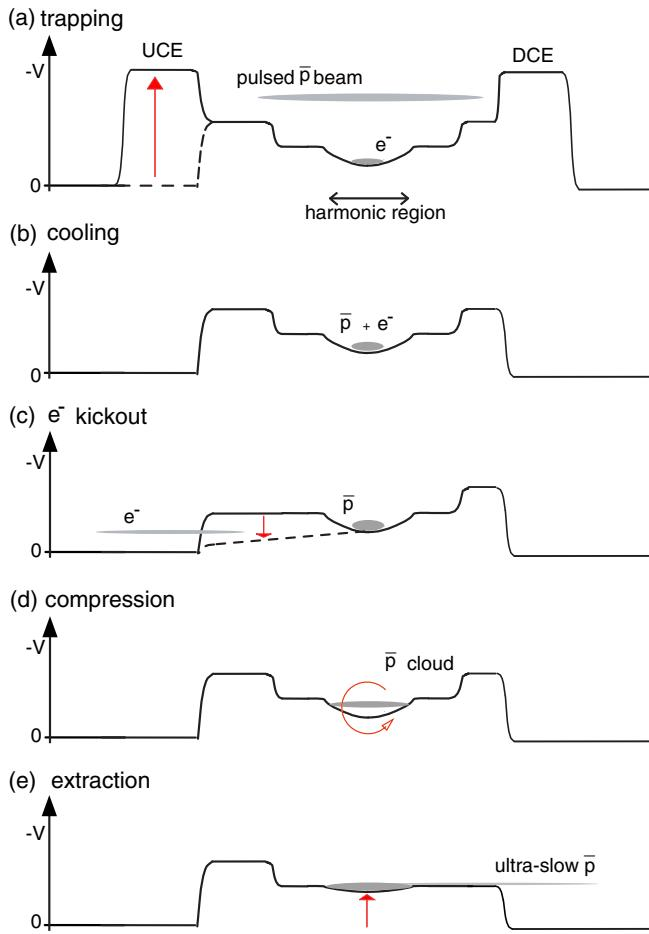
FIG. 8. Antiproton trapping, cooling, electron kick-out, compression, and extraction procedures.
