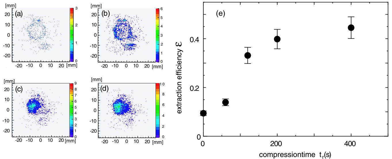
FIG. 16. (a)–(d) The PSD images of extracted  $\bar{p}$  for  $t_r = 0, 60, 120$ , and  $200$  s. (e) The extraction efficiency  $\epsilon$  as a function of the compression time  $t_r$ . The rotation frequency was  $f = 247$  kHz and the peak-to-peak amplitude was  $V_r = 0.56$  V.
