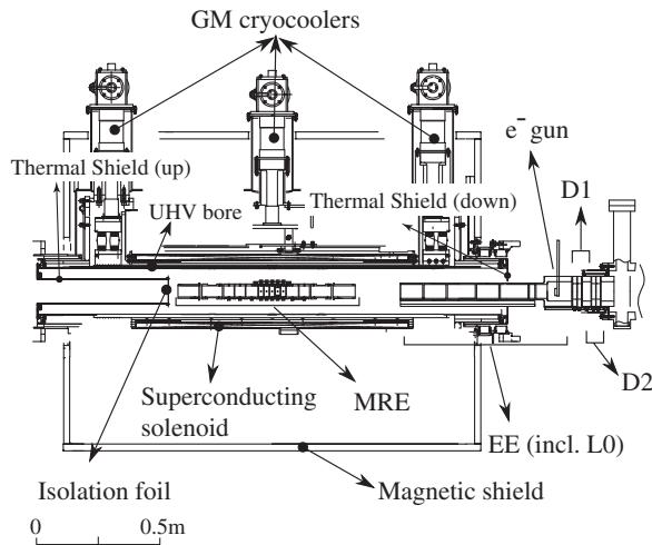
FIG. 2. Cross sectional view of MUSASHI and the ultraslow beam transport line.
