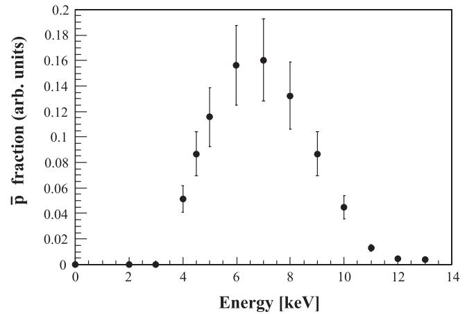
FIG. 13. The energy distribution of 111.5 keV  $\bar{p}$  beam after passage through the foils from the RFQD.
