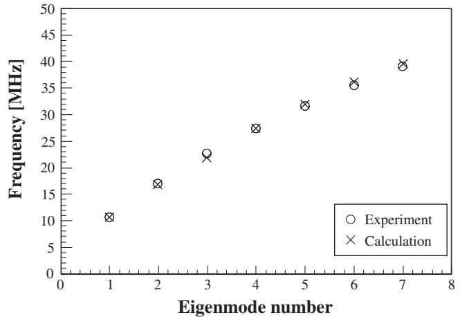
FIG. 7. Observed and calculated axially symmetric frequencies up to 7th eigenmode.
