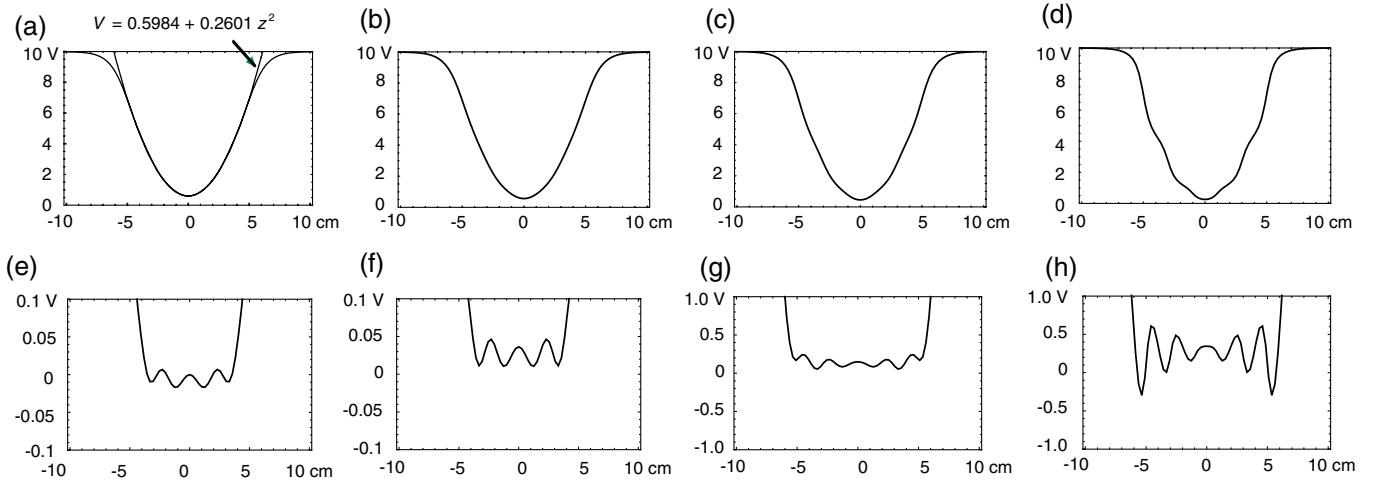
FIG. 5. (a) The potential produced at  $\rho = 0$  mm. A fitting quadratic function is also shown. (e) The difference between the produced potential and the quadratic function in the case of (a). (b) and (f) Potential and difference at  $\rho = 5$  mm, (c) and (g) at  $\rho = 10$  mm, and (d) and (h) at  $\rho = 15$  mm.
