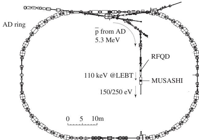
FIG. 1. Scheme of the MUSASHI sequentially combined with the AD, the RFQD, and the LEBT. The AD provides 5.3 MeV antiprotons. The RFQD decelerates them to 110 keV and transports them to the MUSASHI via the LEBT. The antiprotons are trapped and cooled in the MUSASHI, and then extracted at 150 or 250 eV.
