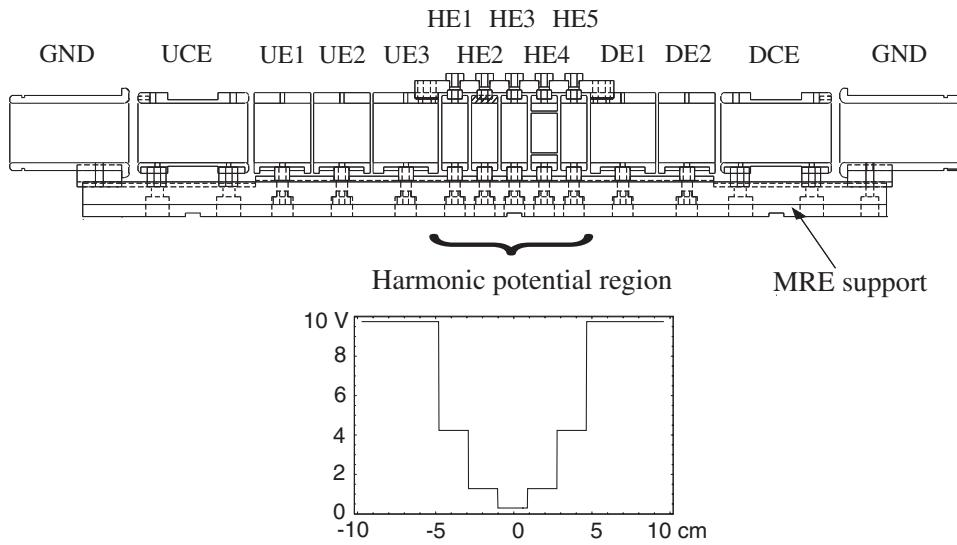
FIG. 4. Configuration of the MRE. The lower part shows the voltages applied on each ring electrode for a harmonic potential well.
