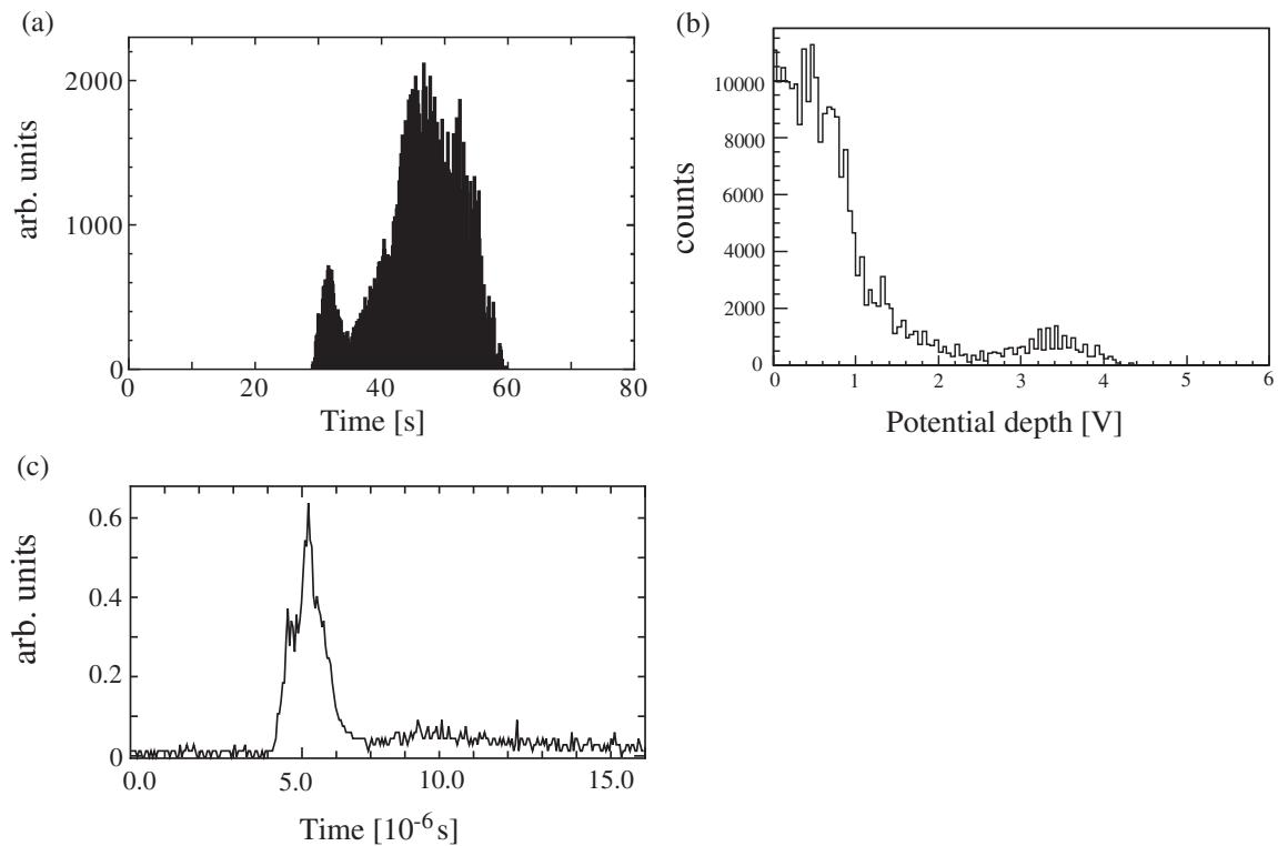
FIG. 17. (a) Typical time profile of extracted  $\bar{p}$  beams for DC extraction. (b) The number of extracted  $\bar{p}$  against potential depth of the MRT. (c) Typical time profile for pulsed extraction.
