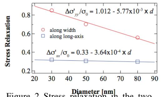
Figure 2 Stress relaxation in the two orthogonal directions.
