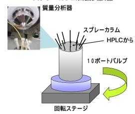
An instrument which coupled with an automatic rotation stage and a ten-port valve (Spray column exchanger).
